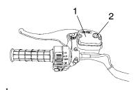
**NOTE:** When checking the fluid level, the ATV must be on level ground with the handlebars straight. If the fluid level is low add DOT 3 brake fluid only. See page 121 for the part numbers of Polaris products.
